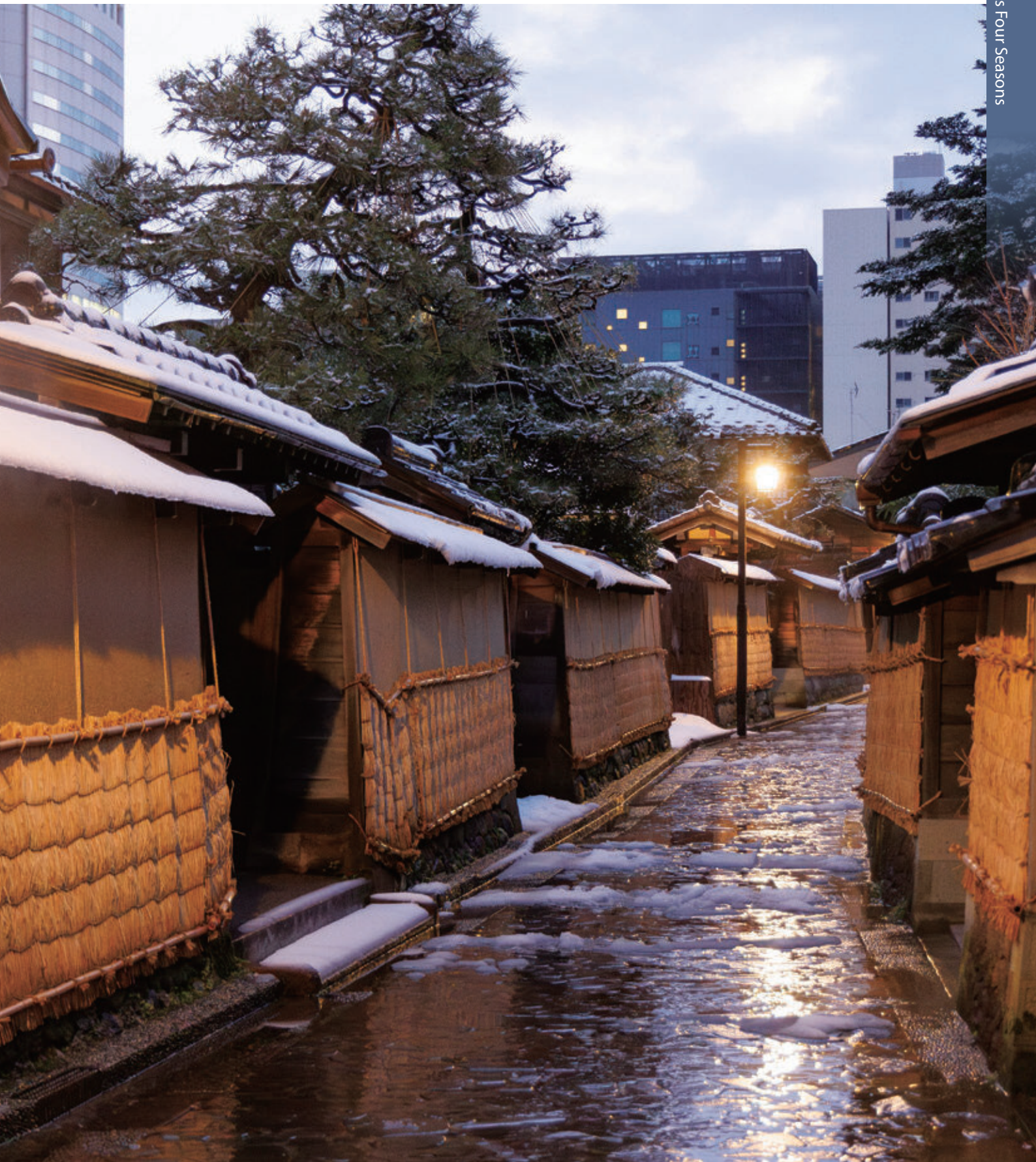
長町武家屋敷群の土塀の藁掛け Woven straw mats on the earthen walls in the Nagamachi samurai residence area
